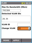
Automatic detection of VLAN ID's allows the user to configure NaviTEK NT for operation on a VLAN.
